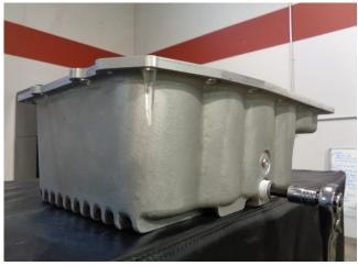
**5.** Inspect and wipe clean the stock oil pan gasket. If the gasket is in good condition, it can be re-used.
