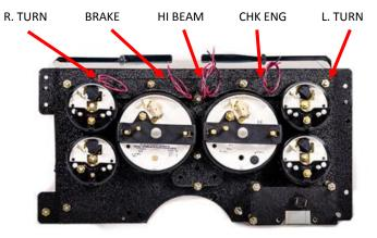
Indicators are LEDs, pre-wired for 12V operation. Red is power black is ground
