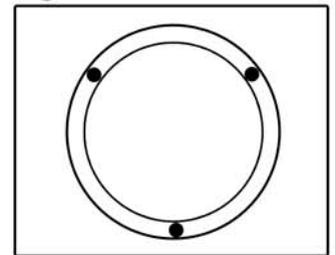
1. Trace Ring 2 on a separate sheet of paper as your template. Hole in floor has to be 2 7/8" diameter (2.875).
