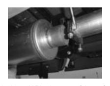
14. Insert Y Pipe into rear of the muffler.
