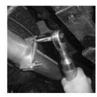
17. Position exhaust clamp over slip connection on tip . Repeat for Left side.
