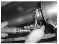
13. Insert muffler into intermediate pipe. Place exhaust clamp with hanger at the front of the muffler. NOTE: Support the muffler temporarily, until the muffler hanger clamp is used.
