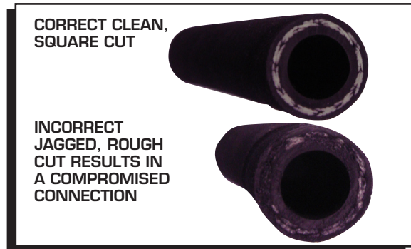
Figure 5 Severing the Hose Properly.
