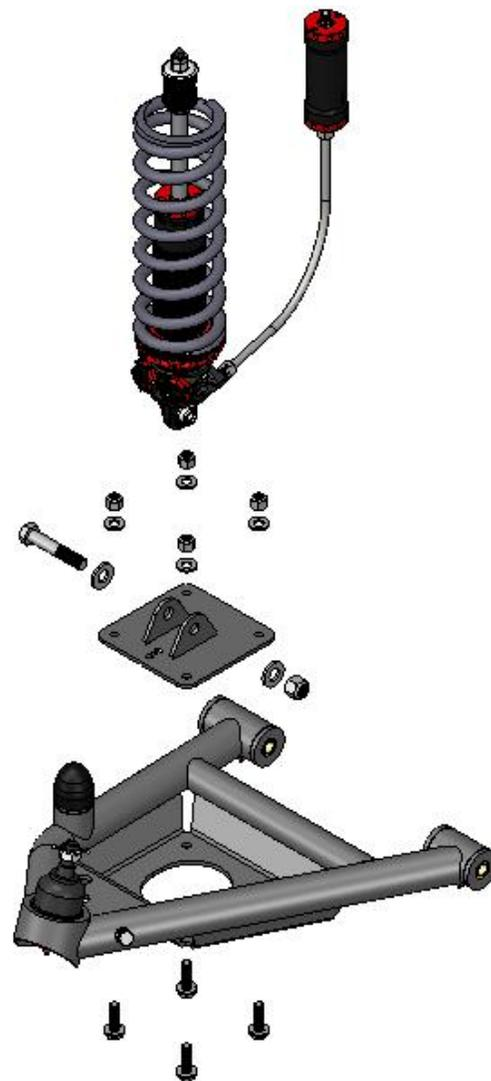
**Note:** Moving the spring seat adjuster will not change the spring rate, only the vehicle ride height.
