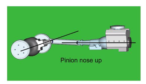
How do you set the pinion angle? On a single-piece shaft you want to set it up where a line drawn through the center of the engine crankshaft or output shaft of the transmission and a line drawn through the center of the pinion are parallel to each other but not the same line.
