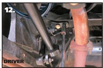
**12.** Swing the tab up to the frame, keeping the linkage straight from side to side. Use the tab to mark the location of the holes that will need to be drilled. Drill the holes with a 3/8" drill bit. Install a 3/8" flat washer on each of (2) 3/8"-16 x 1 1/4" hex bolts and install them through the bracket and drilled holes. Install a 3/8" flat washer & 3/8"-16 nylok nut on each bolts sticking through the frame. Torque the hardware and repeat on the other side.
