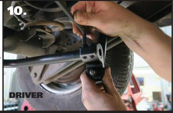
**10.** Apply Antisieze to (4) 3/8"-16 x 7/8" Socket Head Cap Screws and thread them into the Clamp-On Ends. Install a clamp-on end on each end of the bar. The End Link mounting hole should be mounted to the outside of the bar and pointing down. Start with the mount flush with the end of the bar.
