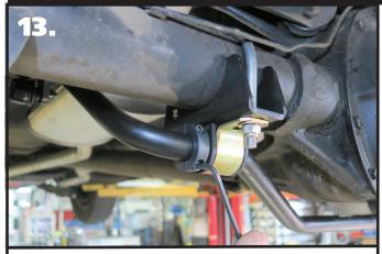
**13.** Install the locking rings on the outside of each bushing assembly. Use a hex key to take the locking ring apart. Reassemble it on the bar positioned next to the outside of the bushing assembly. Push the locking ring up against the bushing assembly and tighten.
