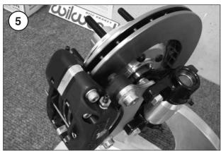
6) Install caliper on caliper bracket as shown. Use Loctite on bolt threads, torque to 30 ft lbs.
