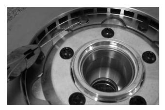
3) Install rotor onto adapter plate (verify that beveled ID of rotor lugs face toward the adapter plate and that rotor is seated squarely on adapter). Install bolts and torque to 15 ft lbs, secure with lockwire.
