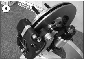
8) Verify that hub and rotor spin freely with no interference or contact with caliper (refer to step 7 and re-shim if required). Insert brake pads into caliper and secure with pin.
