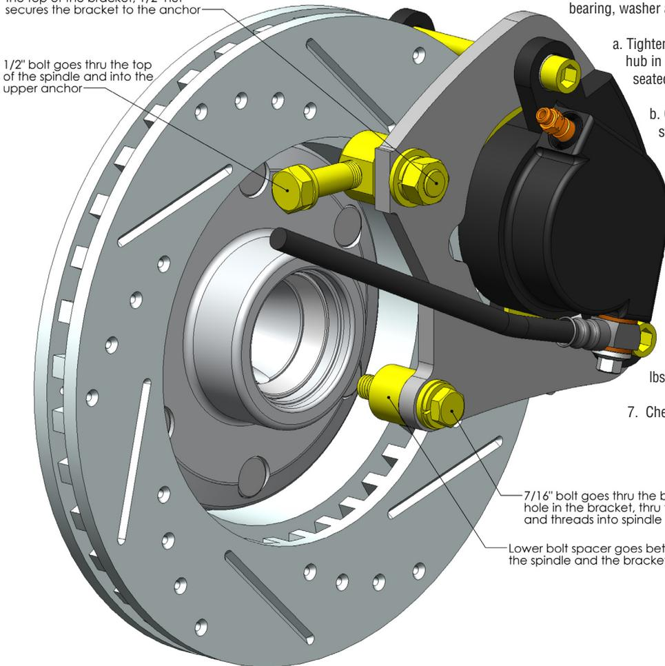
7/16" bolt goes thru the bottom bolt hole in the bracket, thru the spacer, and threads into spindle
