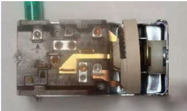
**NOTE 1:** If you are using this new AAW switch in a 1953-55 Ford Truck that originally used a 6 volt switch, you will find that the threaded area on your original nut is too small in diameter. You will need to purchase a new 1956 12 volt style replacement nut which is larger in diameter and will fit this new AAW switch and still allow for the use of your stock dash bezel. These are readily available from your favorite truck parts supplier.
