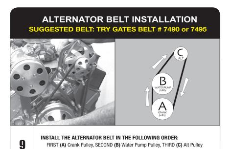
ADJUST the tension, tighten all the bolts and check for proper alignment.
