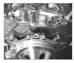
REMOVE the 2 upper water pump bolts.
