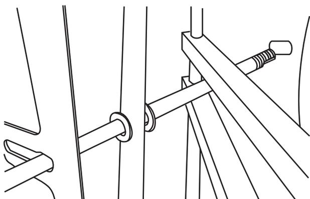
**3** Insert steering shaft through hole in the top body panel.
