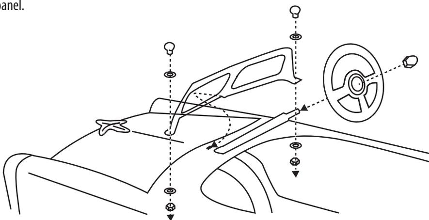
**5** Assemble windshield and steering wheel as shown
