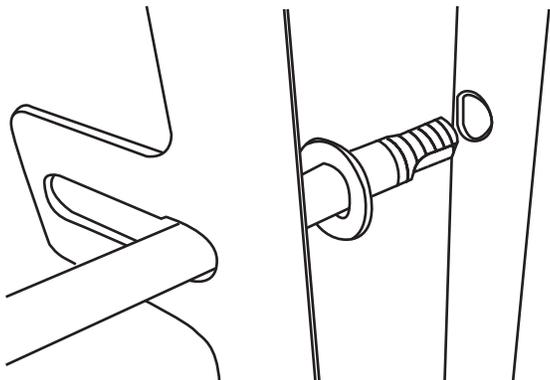
**1** Turn the car on its right side on a soft surface to protect the finish. Partially insert the steering shaft through the slot in the front crossmember and install one washer before inserting the shaft into hole in the frame.
