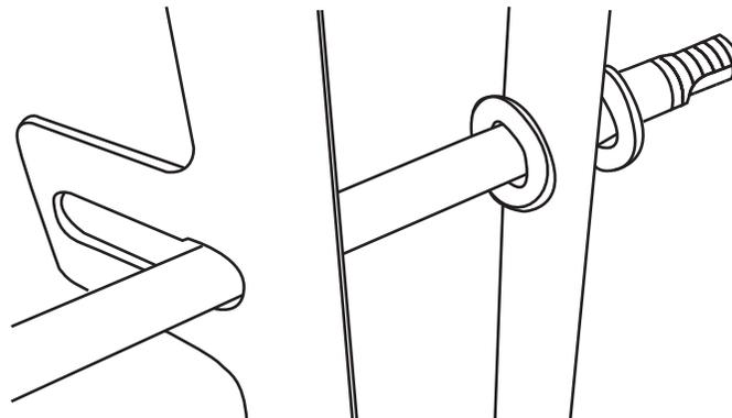
**2** Insert steering shaft through hole in the frame and install second washer.
