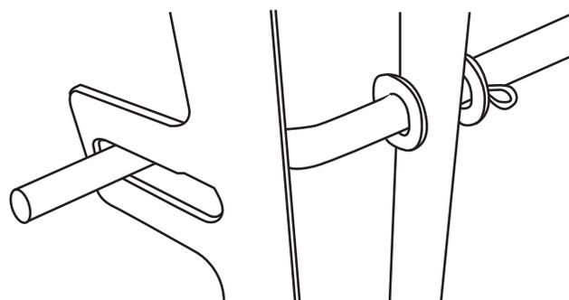
**4** Insert cotter pin into pre-drilled hole in steering shaft to locate and retain shaft.
